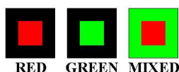
Fig. 1. Landmarks used in MRSCL Geometry. The inner and outer color square design was chosen for the robot to achieve a robust visual detection.
