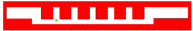
(b) Situation after the robot moves out of the corridor. The robot is localized. The number of particles is reduced to 80.
