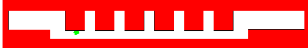
(b) Situation after 50 iterations of the algorithm. The robot is localized. The number of particles is reduced to 80.
