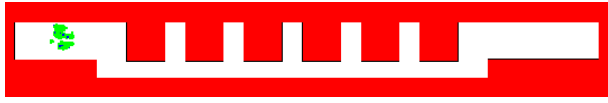
(a) Situation after 7 iterations of the algorithm. The robot pose is limited to a small area within the environment. The number of particles is reduced to 900.
