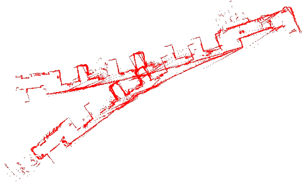
FIG. 9. Map of the Computer Science Department, at Universidad Catolica de Chile, obtained from raw data. The true area possesses only one corridor.
