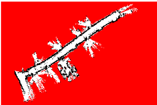
FIG. 7. Map of Wean Hall, at Carnegie Mellon University, obtained from proposed main algorithm, and IS sample size n = 10 .
