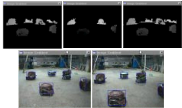
Figure 10. Upper images show the structures detected by the stereo agent at some points during the robot motion. Lower images show the detection of the obstacles for the initial and final frame in the video sequence using information from the color and the stereo agents.
